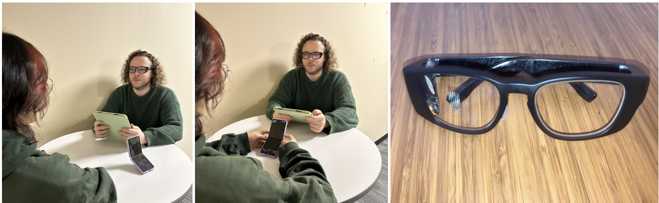
Figure 1: Left: Hearing participant cannot see captions. Center: Hearing participant can see captions. Right: tooz DevKit head-worn display.
